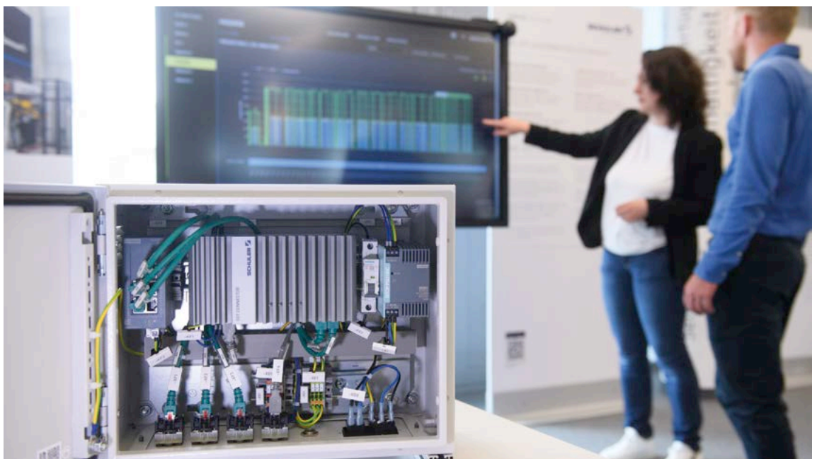
Edge in a box: All the system hardware is assembled in a cabinet that is easily installed by the user and then activated remotely by Schuler. “Schuler solution for Industrial Edge”
