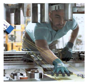
Visual Die Protection detects foreign objects or other sources of danger in real time and stops the line before any damage occurs.
